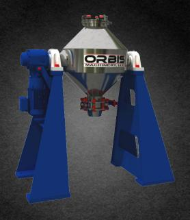
Blending in its simplest form is the combining of two or more materials to produce a homogeneous mixture. Normal tumble blending of free flowing materials provides a gentle mixing action. We offer two types of tumble blenders.
