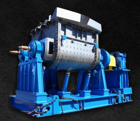
Orbis Machinery custom-designs and engineers Double Arm Mixers and Mixer Extruders for shearing and kneading high viscosity products.
