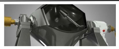
With a smooth internal finish, complete discharge and elimination of cross batch contamination are realized. Orbis Machinery Cone Tumble Dryers (CTD) can be designed for up to 500° F jacket temperatures and high vacuum. For superior drying, mixing and ease of cleaning the Orbis Machinery CTD is the dryer of choice.
